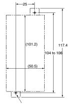
M4 tapping screws provided. Approximate pilot hole dimensions: Panel thickness of 0.8 to 1.2 mm: 3.6 mm dia. Panel thickness of 1.6 to 4.0 mm: 3.7 mm dia.
